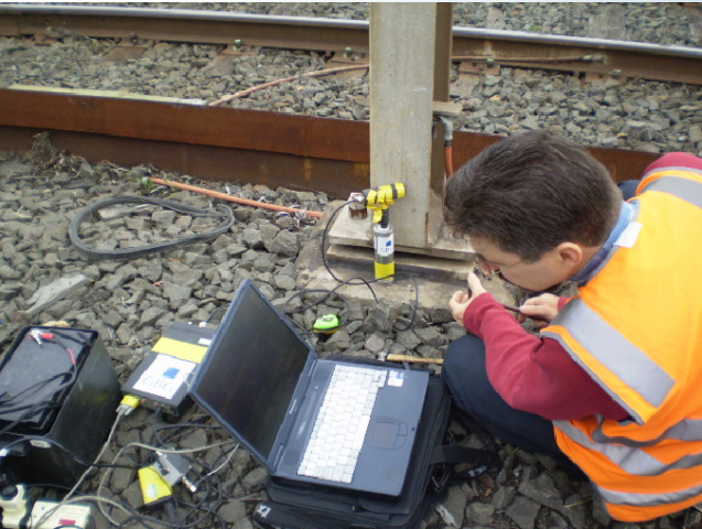
FIGURE 1: IMPACT ECHO EQUIPMENT BEING USED TO MEASURE FOOTING DEPTH.
